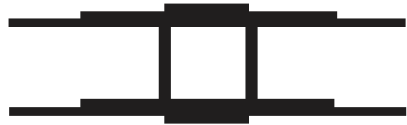
Fig. 1. Wide band conventional branch line coupler with dual quarter wavelength lines in each port
